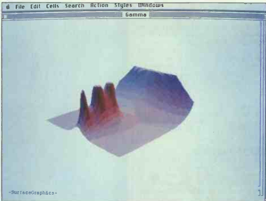
Surface: Another memory eater — this single graphic takes up just over 1Mbyte but shows the excellent results that can be obtained. The surface is illuminated using Mathematica's default settings of no ambient light and three point sources (red, green and blue) at 45° to each other
