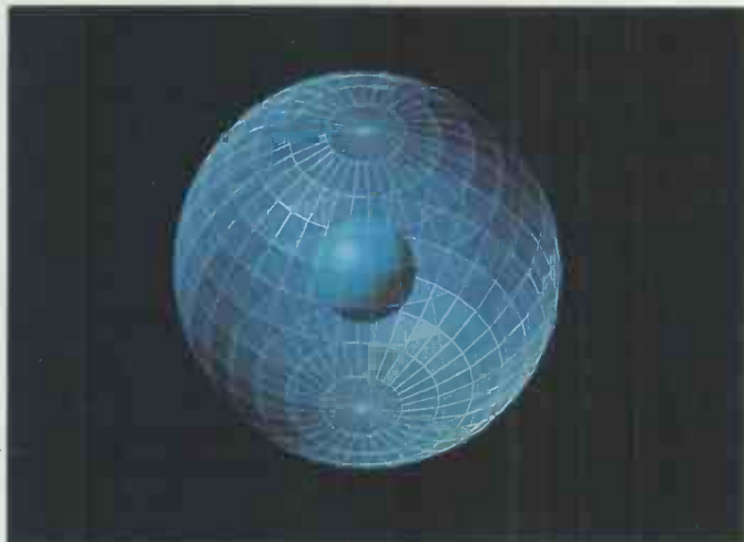
A high-resolution synthesised image showing extensive use of Giraud shading, texturing and specular reflection
