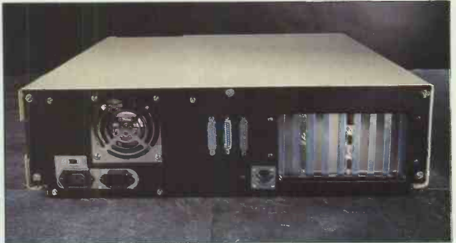
The rear shows the Hi-Grade's twin serial ports, and its TTL and analogue VGA video outlets
