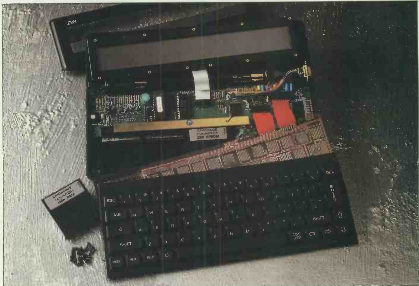
The most impressive component of the Z88 is the 'dead-flesh' keyboard (which is quiet in operation). The electronics are contained in a thin, plastic film, and are activated when your fingers touch them through the rubber mat
