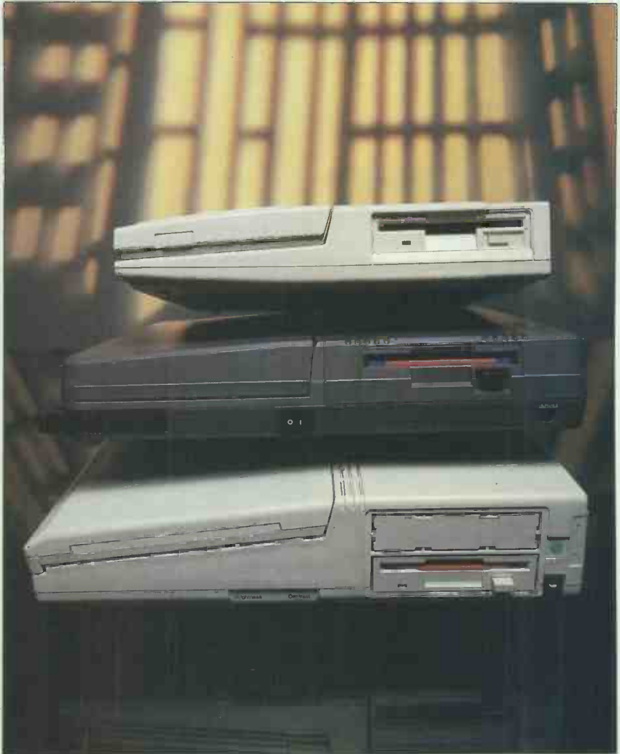
All three machines feature 720k 3½in disk drives, and as this format appears on IBM's entire PS/2 range, there should be no shortage of software. The Spark and the PC-4501A can be fitted with second internal drives, but in the T1000 DOS in ROM means that one drive is adequate
