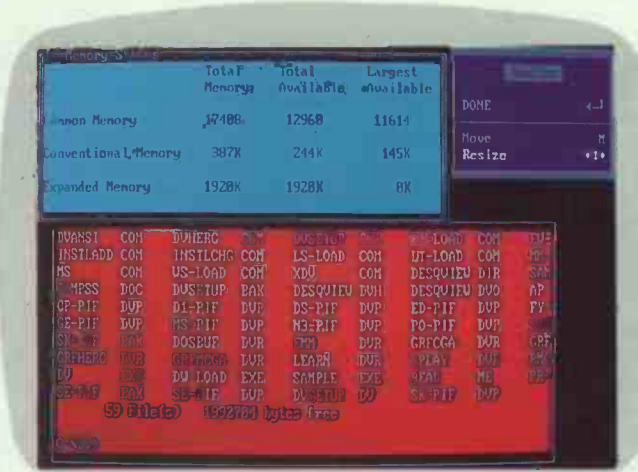
DESQview has a few applications available immediately before any new ones are installed. Shown here are the memory display (being resized), a DOS window and the rearranged sub-menu of DESQview
