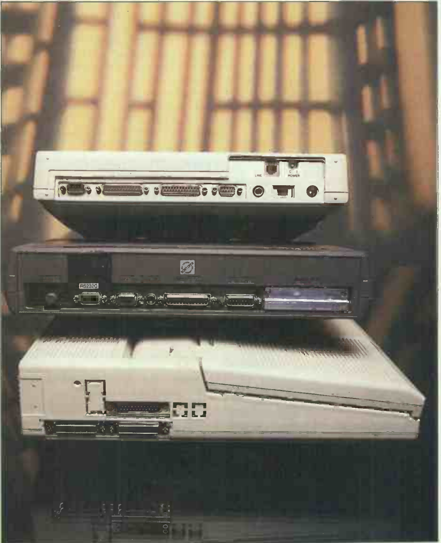
The Toshiba T1000 and the Datavue Spark have identical ports at the rear, consisting of serial port, parallel port, RGB, external floppy disk and composite video. The Sharp PC-4501A has only a serial port, a parallel port and an external floppy disk mounted on its right-hand side
