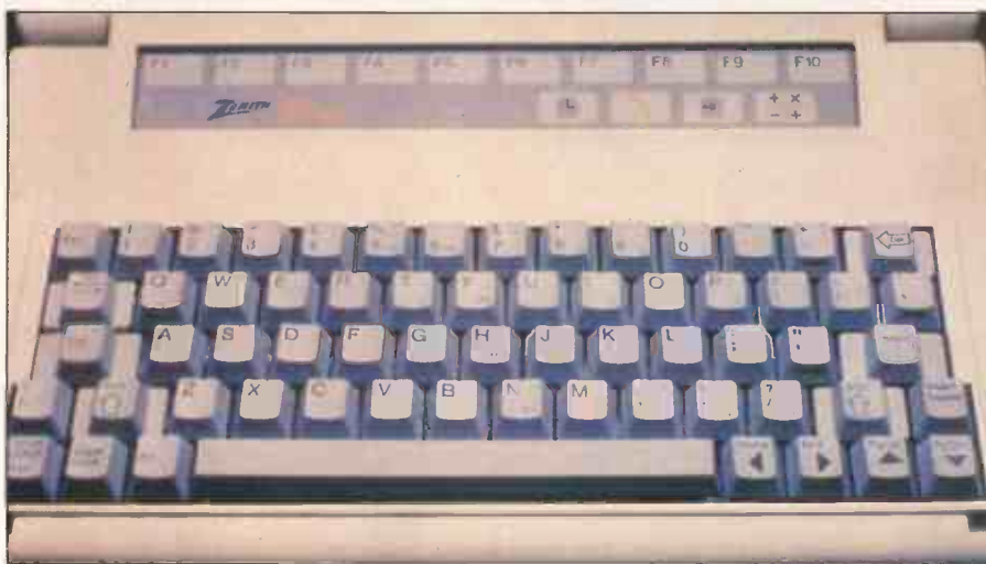
The Pivot Two's American keyboard is built into the box
