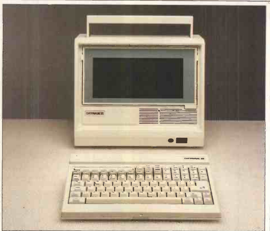
The Quadram Datavue: a detachable keyboard and upside-down disk drive
