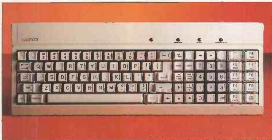
The F10's membrane keyboard looks and feels like a traditional unit
