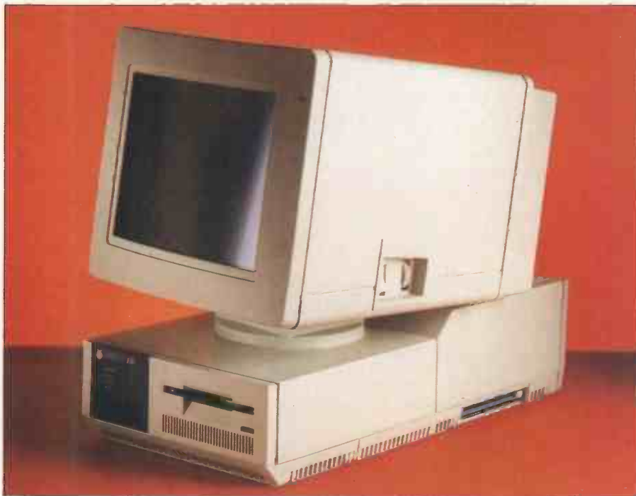
There is no metal shield between the monitor and the system box
