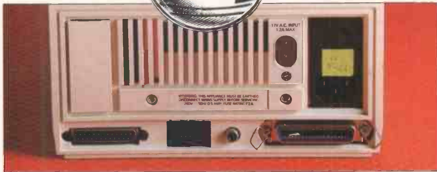
The back features a two-pin monochrome monitor socket
