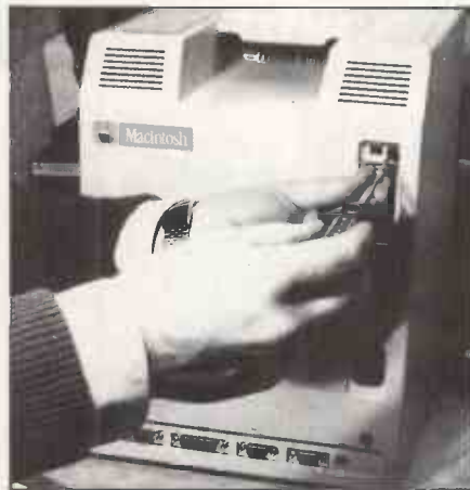
Figs 3a-3c The position of the five Allen screws which hold on the back of the Macintosh
