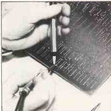
Fig 7 Sucking the solder from the same side of the board as the iron
