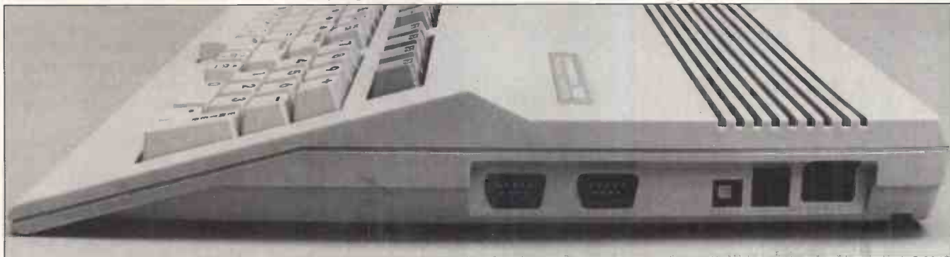
View from the side: two standard joystick ports, the reset button and power on/off
