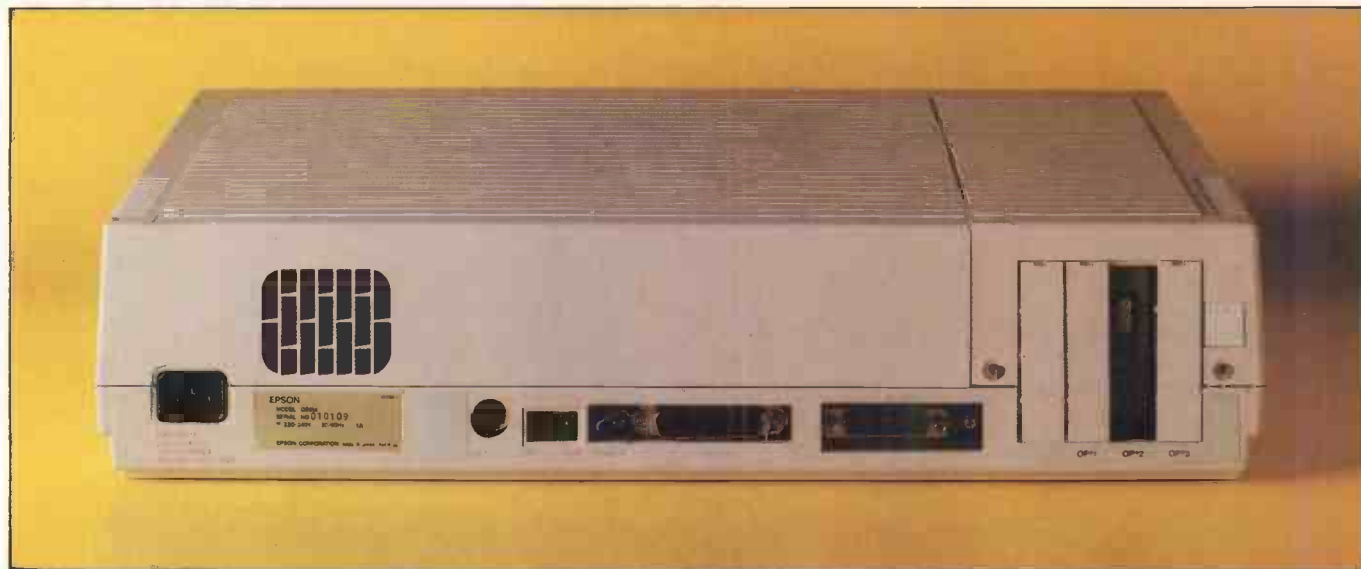
The rear panel has space for four expansion cards but the PCB will only support three
