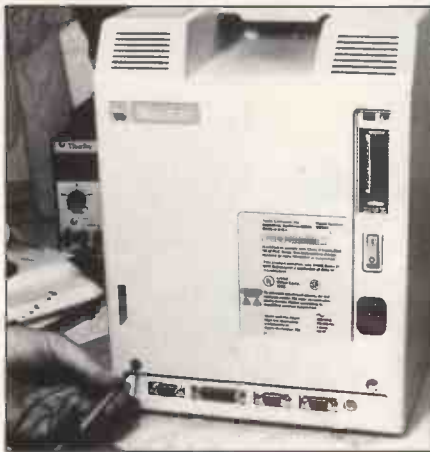
Figs 3a-3c The position of the five Allen screws which hold on the back of the Macintosh
