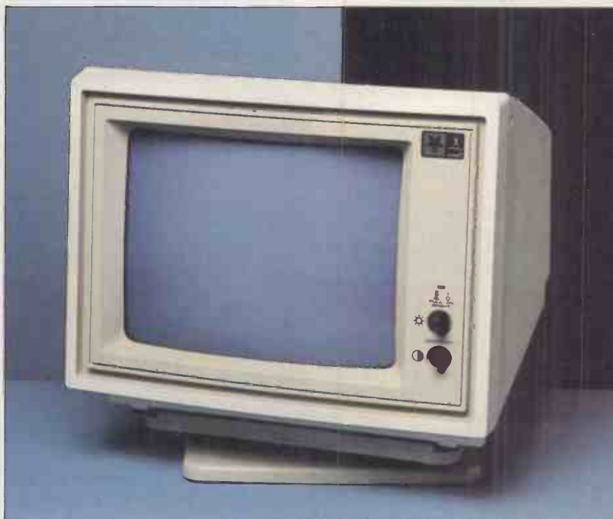
The standard monochrome/green monitor has brightness and contrast controls
