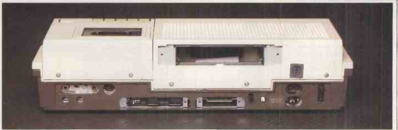
Unscrewing three panels reveals the disk interface slots, external DIP switches and standard joystick ports
