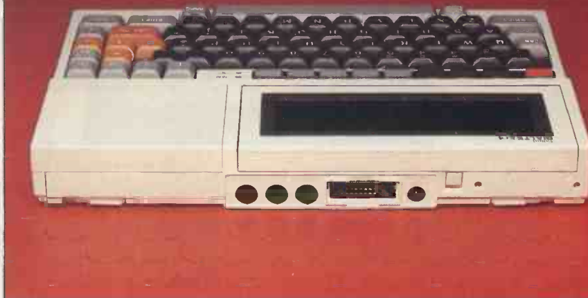
A 20-way connector on the back functions as a Centronics port
