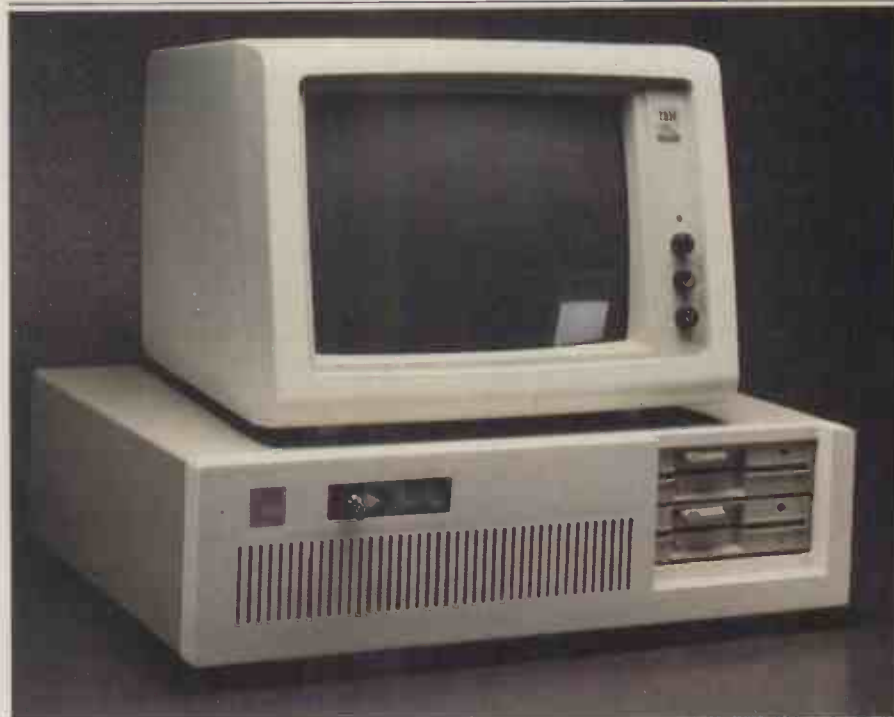
On the right two half height 5¼in floppy disk drives
