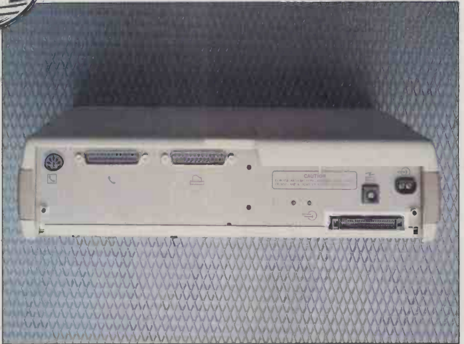
Internal modem output, two RS232s, the system expansion bus and two power inputs
