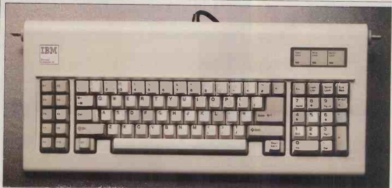
The PCAT keyboard is a great improvement on the PC — the typing areas are well spaced and the RETURN and shift keys are larger.
