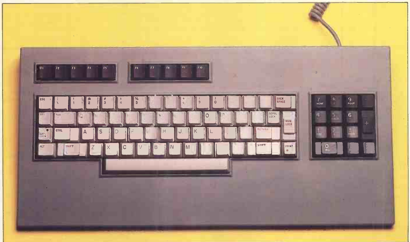
A major departure from the IBM standard: function keys are well clear of the main typing area
