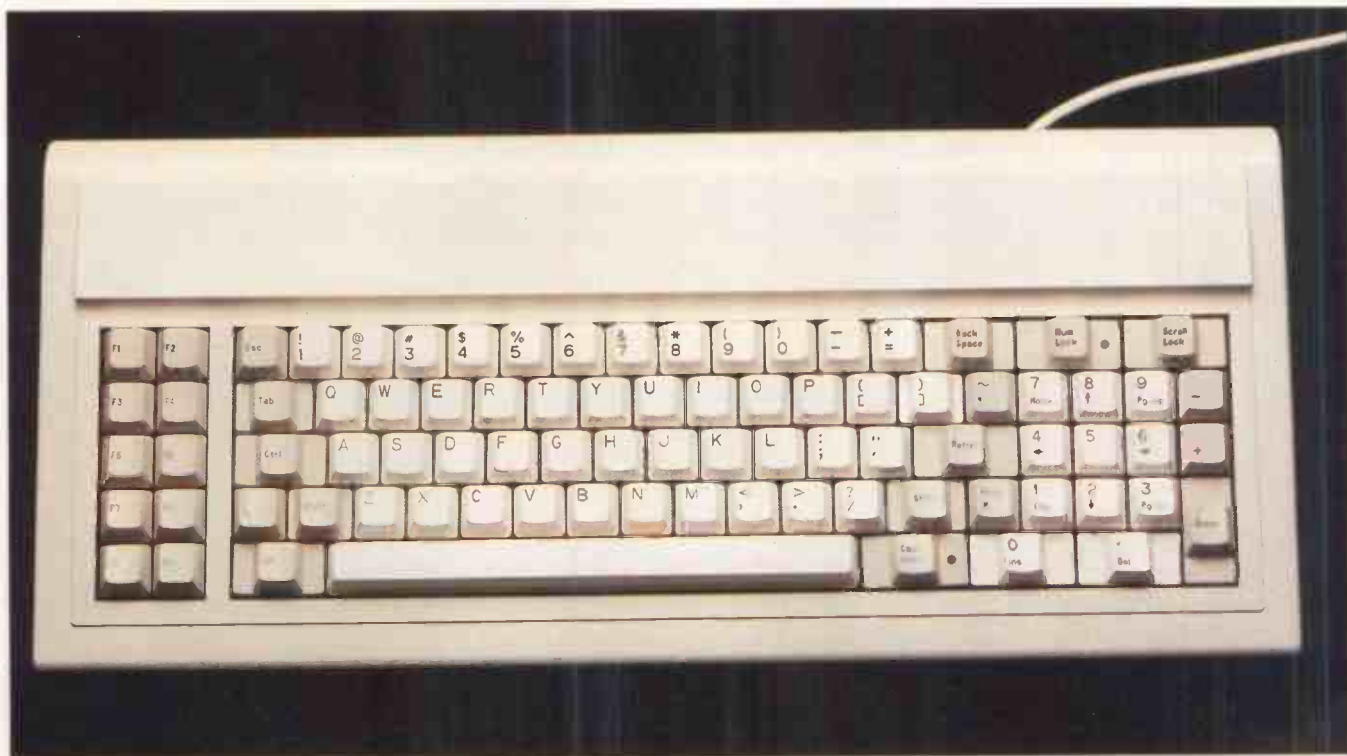
Average IBM PC clone keyboard, although the Caps Lock and NUM Lock keys with built-in LEDs are innovative
