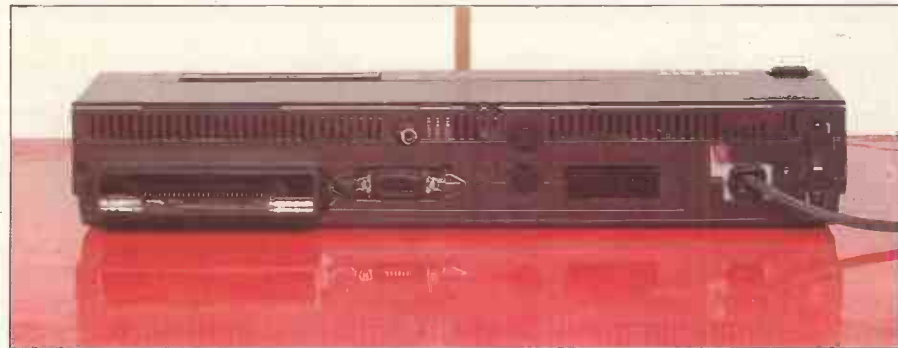
At the rear an impressive array of video outputs together with cassette interface
