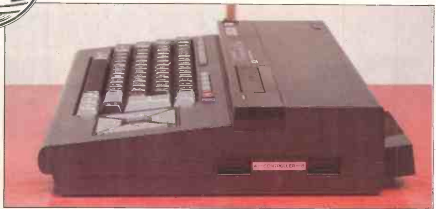
A side profile shows the ports for two joysticks
