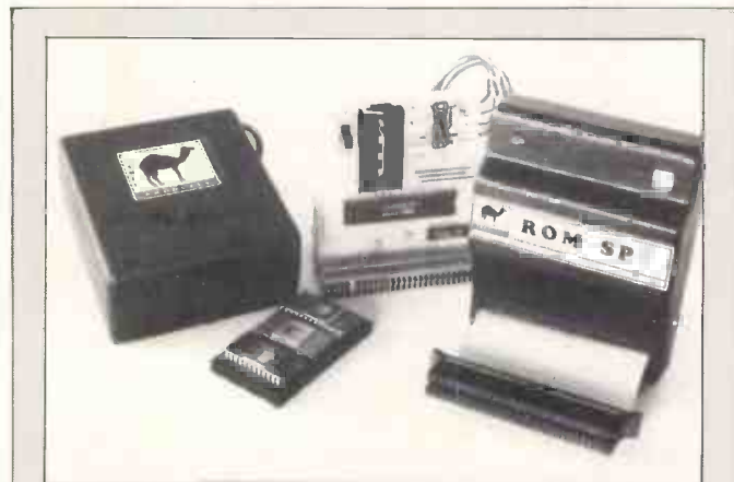
A camel for the Spectrum — nothing to do with Jeff Minter's hump-mania, either. It's a family of devices to load EPROM memory chips with your own program, run the program, and change the program. The unusual feature, according to Cambridge Micro Electronics (CaME1), is that you can use the Spectrum ROM program memory at the same time.
