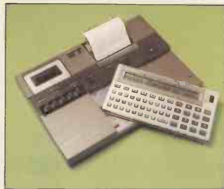
Computer slots neatly into cradle.
