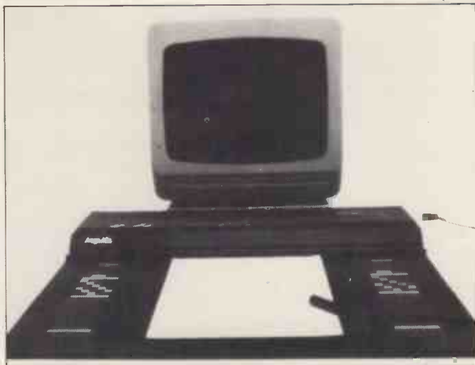
This is a pad on which you write, and a screen on which you read what the computer thought you wrote.
