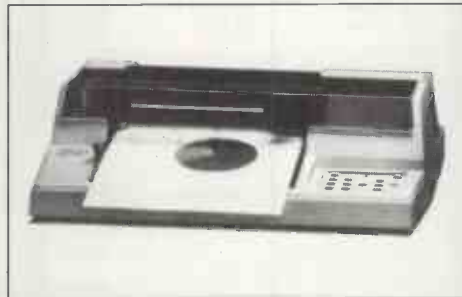
HP 7470 low-cost plotter, for full-colour hard-copy charts or overhead transparencies.
