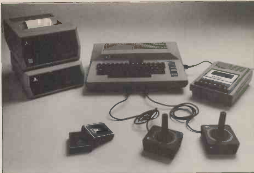
A useful configuration comprising an Atari 800 with disk drive, forty column printer, cassette recorder and a couple of joysticks.
