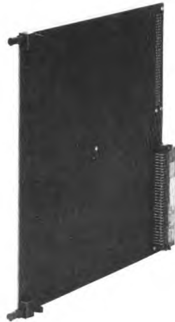
FIG. 16—Eight-unit plug-in-unit showing card locks
