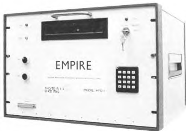
Fig. 2—Prototype electronic multipurpose programmable information recording equipment (EMPIRE)
