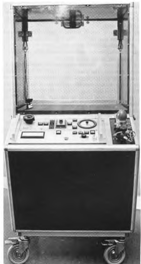
FIG. 5—The BPO impulse generator
