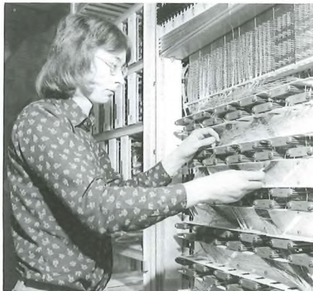
FIG. 8—Cyclic-store data-threading field
