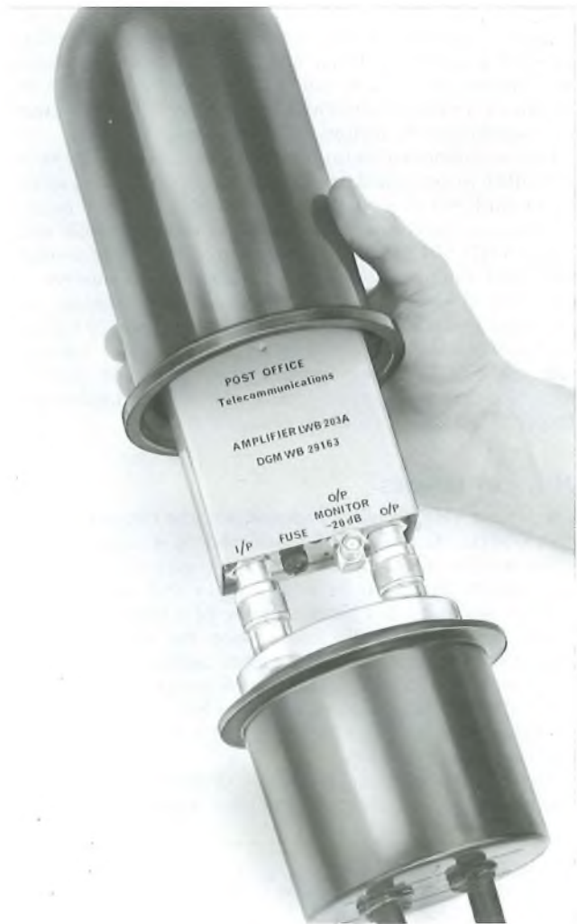
FIG. 4—Third-generation VHF-UHF amplifier in Sleeve No. 31A
