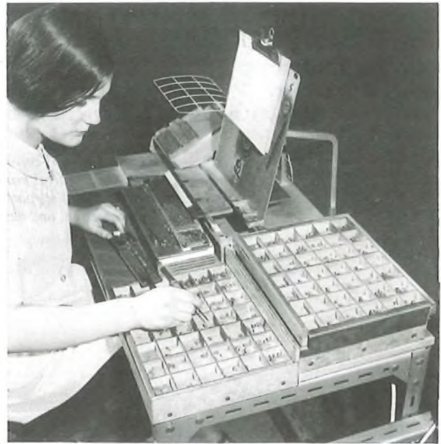
FIG. 9—Setter making-up a legend
