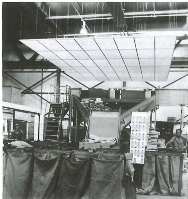
Diffuser suspended over the concentrator's working area
