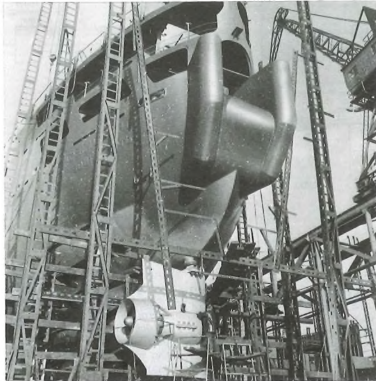
Fig. 1—Stern of CS Monarch with power rudder fitted, shortly before the launch date
