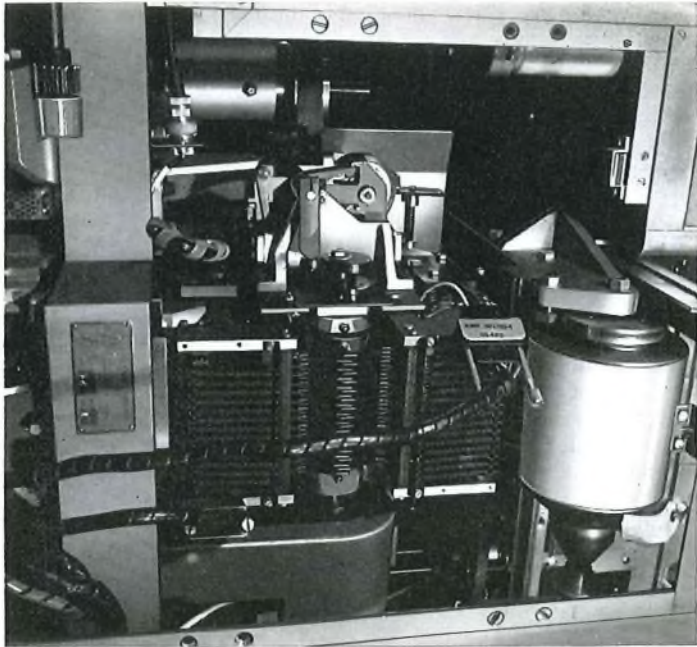
FIG. 11—T-type code-printer unit
