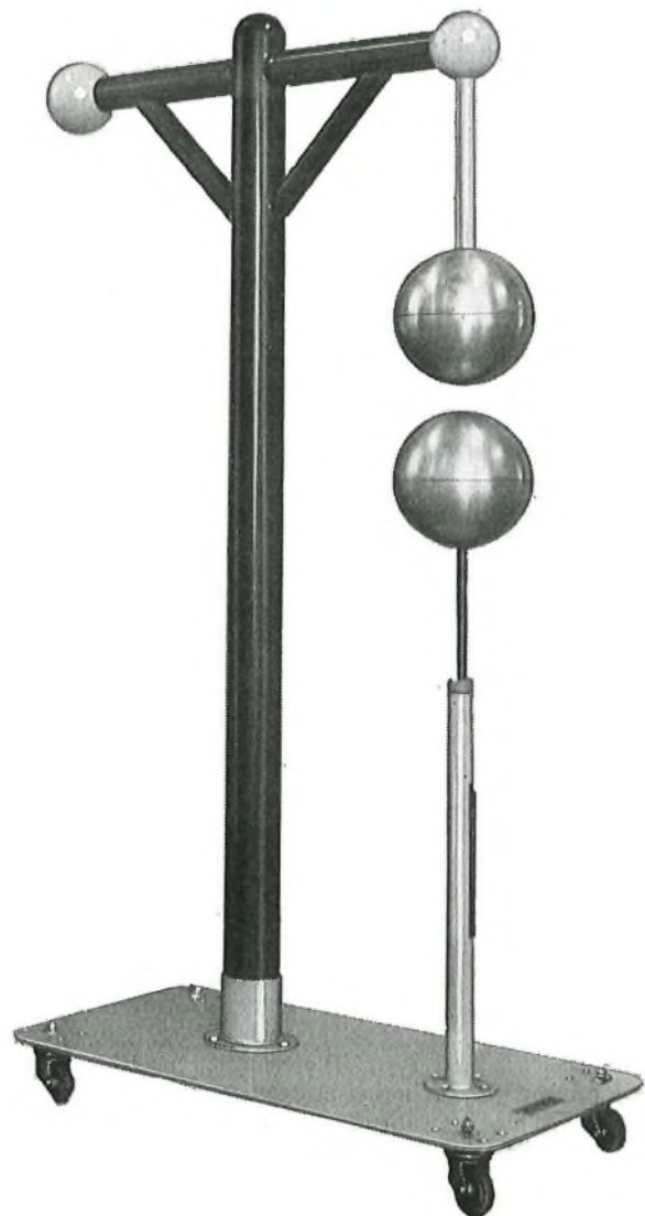
FIG. 4—Adjustable sphere gap
