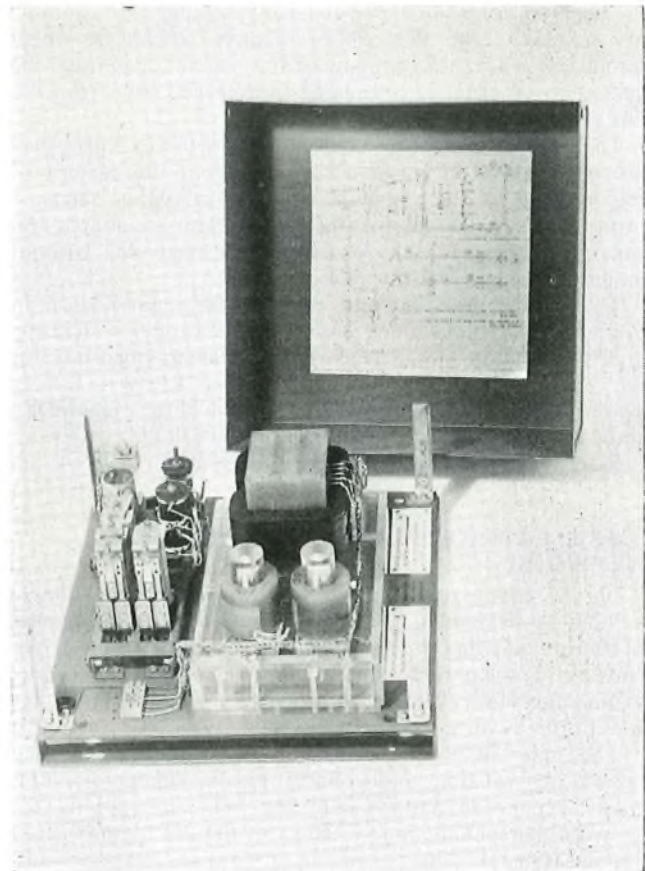
FIG. 2—Line Isolating Unit 1A
