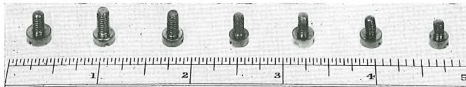
FIG. 2—RANGE OF 4BA AND 5BA SCREWS REQUIRED TO BE SELECTED
