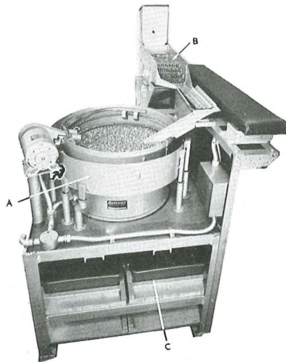
A—Second sorting unit B—Filling hopper and linear feeder C—Tray for sorted screws FIG. 1—SCREW-SORTING MACHINE
