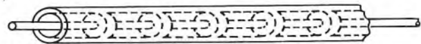
(d) Stage 4: Construction Completed; Inner Conductor contained in Centre of Inner Tube
