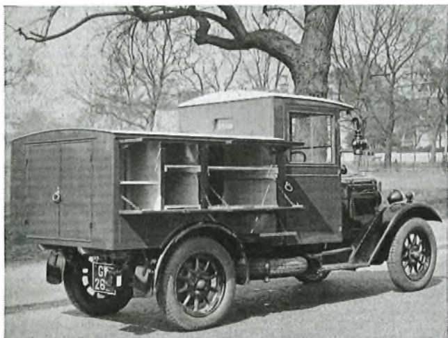
FIG. 1—1932 15 CWT VEHICLE DESIGNED FOR SUBSCRIBERS' APPARATUS INSTALLATION DUTIES
