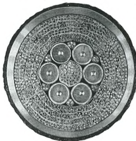
6-tube Type 375 PWDI Coaxial Cable with additional layers of V.F. pairs
