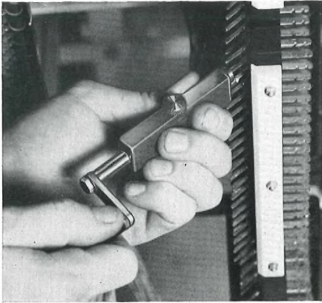
FIG. 7—HAND WRAPPING TOOL BEING USED ON CONNEXION STRIP WITH ANGLED TAGS
