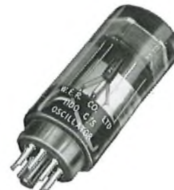
This fixed frequency oscillator is constructed on a standard octal base and encapsulated in epoxy resin.
