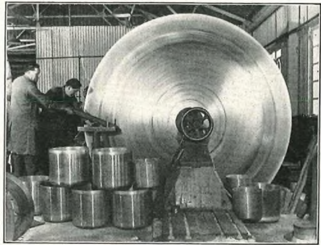
FIG. 12.—SPINNING A 12-FT DISH.
