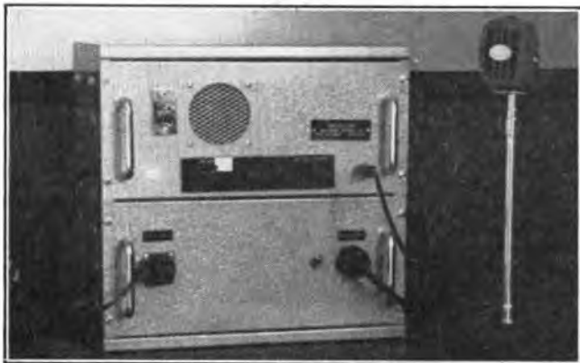
THE FIXED STATION; THE UPPER UNIT IS THE TRANSMITTER AND RECEIVER; THE LOWER UNIT CONTAINS THE POWER PACK.
