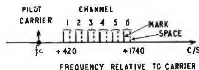
FIG. 6.—ARRANGEMENT OF CHANNELS FOR MULTI-CHANNEL V.F. TELEGRAPH TWO-TONE SYSTEM.
