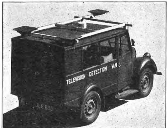
FIG. 2.—THE DETECTION VAN, SHOWING LOOP AERIALS ON ROOF.
