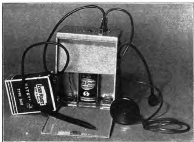
FIG. 2.—THE AMPLIFIER WITH PROBE AND RECEIVER.
