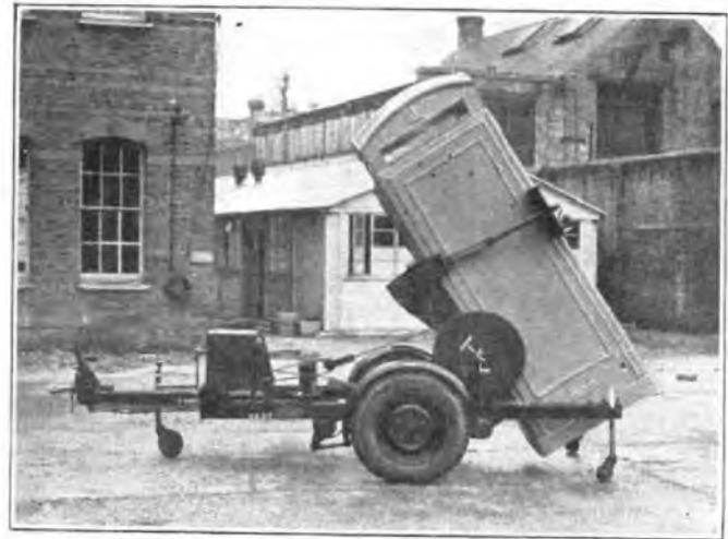
FIG. 2.—KIOSK LIFTED AND BEING TURNED.
