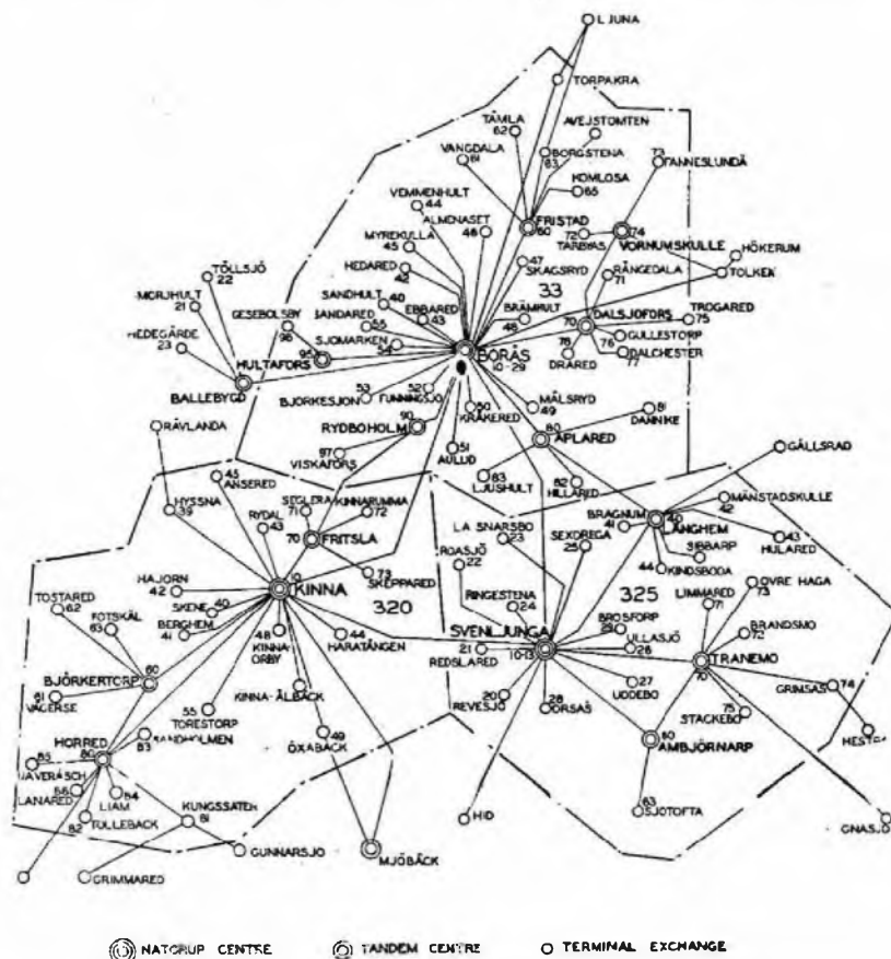
FIG. 1.—ARRANGEMENTS FOR INTER-DIALLING BETWEEN 3 GROUP CENTRES.
