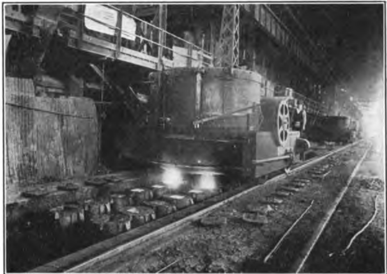
FIG. 6.—FILLING THE MOULDS FROM THE LADLE.
