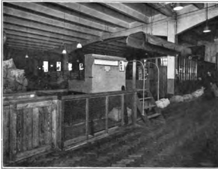
FIG. 2.—WEIGHING MACHINE (GUARD IN "UP" POSITION).
