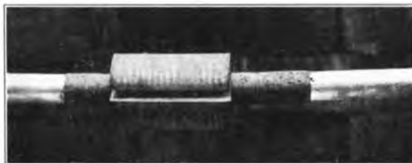
FIG. 3.—ADDITION OF SPLIT RUBBER SLEEVE.
