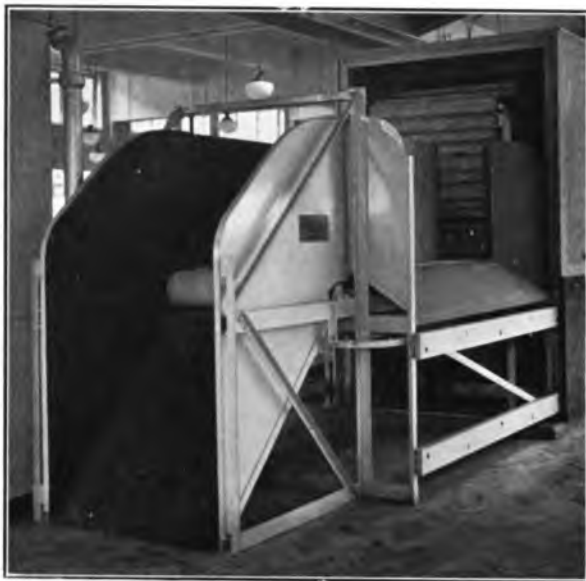
FIG. 9.—DISCHARGE HEAD OF INWARD PARCEL AND BAG CONVEYOR.
