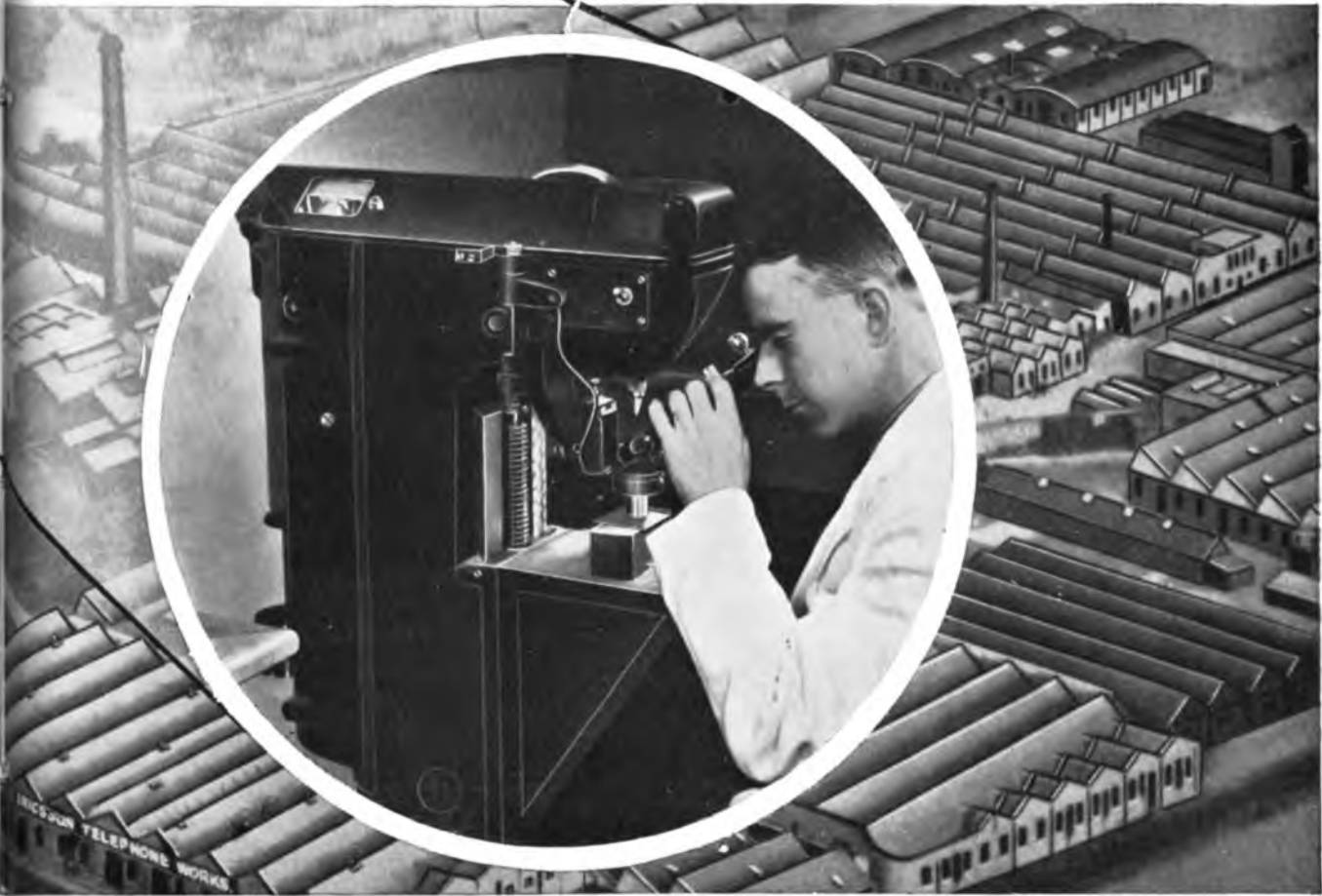
2. Testing the hardness of materials.
