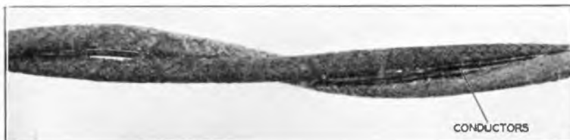
FIG. 5.—INSULATED WIRES DAMAGED BY LIGHTNING.
