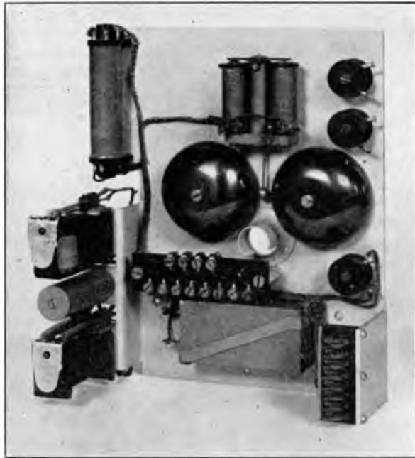
FIG. 3.—BELL SET FOR MANUAL C.B. SYSTEM.
