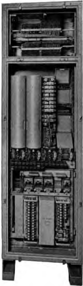
B.P.O. Unit Auto No. 12A 25/100 lines capacity.
