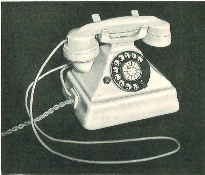
FIG. 3.—DESK TELEPHONE FITTED WITH PUSH BUTTON.
