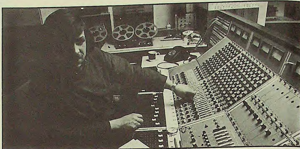
Neil Ross of the REL Studio. The desk is being converted from 16/8 to 20/16.
