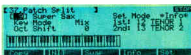
Our state-of-the-art 240x60 dot LCD display lets you view all the parameters while editing.
