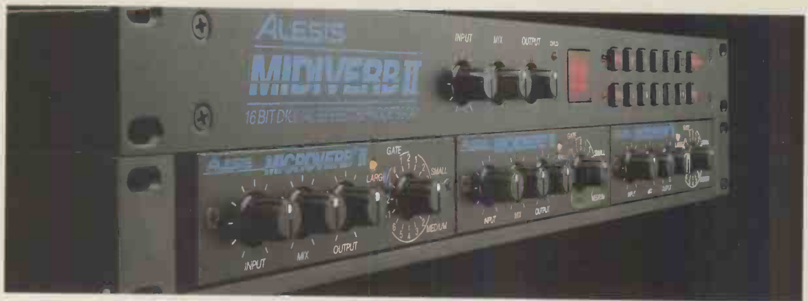
THE MIDIVERB II 16 bit linear PCM stereo effects processor
