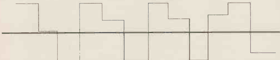
Figure 3B. . . results in an alias frequency lower than the original.
