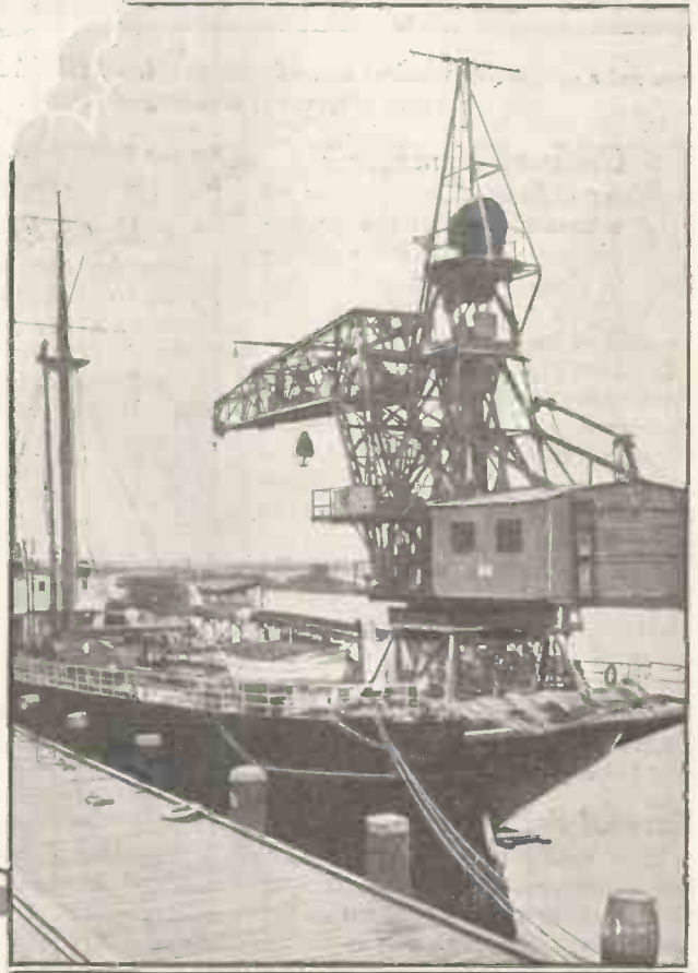
The giant crane on the stern of the "Westfalen" is shown in the photograph above, and the main aerial system can also be seen. To the left are the short- and long-wave transmitters which will work over ranges of 15-90 metres and 500-3,000 metres respectively.
