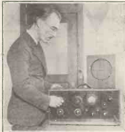
R. L. Knowles, the American inventor, with an ingenious oscillator which he has designed. It produces musical notes which he claims will attract mosquitos, and enable them to be exterminated.
