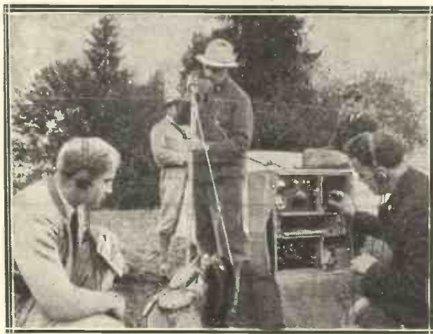
The German-Austrian Alpine Club have obtained two portable combined transmitters and receivers to aid them when search parties have to be sent out. One set, shown in our photo, is left in the valley, while the other is taken along by the searchers.
