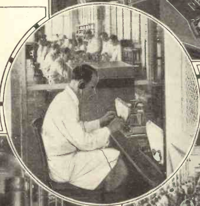
(Below) A section of a big German radio factory showing constructors working in front of a slow-moving conveyor band which facilitates their work.
