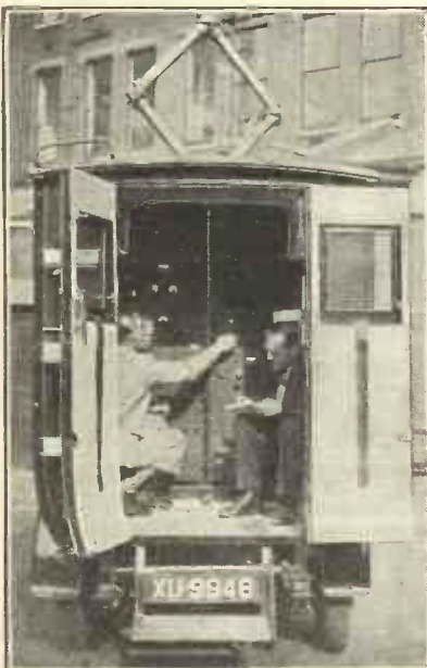
The Post Office officials make full use of the directional properties of frame aerials in their detector vans.
