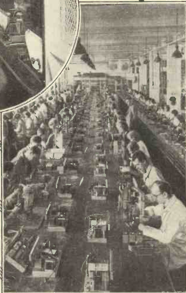
(Below) A section of a big German radio factory showing constructors working in front of a slow-moving conveyor band which facilitates their work.
