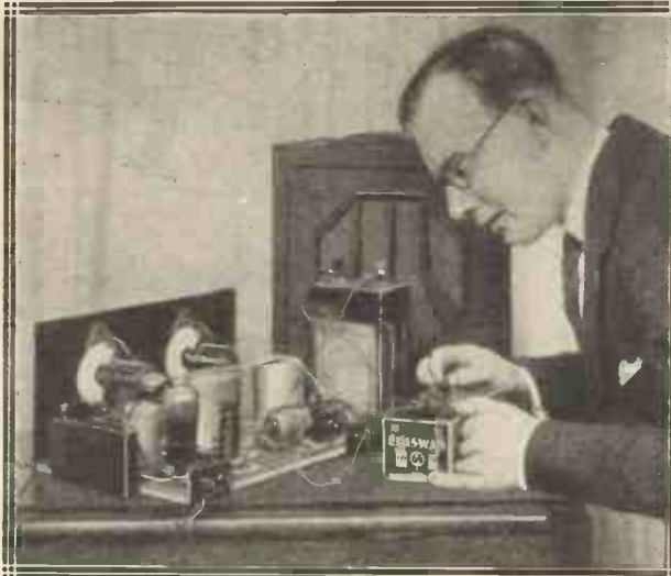
Varying the voltages applied to the three H.T. positive taps will often produce improvements in results. So don't miss this chance of making a fine set even better!
