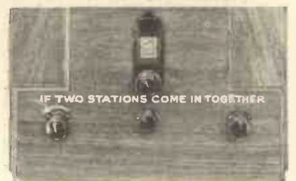
The aerial series condenser provides varying degrees of selectivity, from the cutting-out of the powerful local station to the easy obtaining of a weak but uninterfered-with foreigner.
