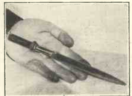
Lead tubing and rubber give the file an excellent "grip."
