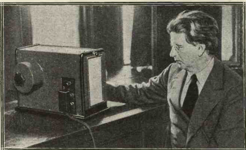
John L. Baird, British pioneer of television, with the latest model "Televisor" which he has prepared now that the B.B.C. is sending out regular television programmes. It is an all-mains apparatus, extremely compact, and with a larger viewing screen than the previous models.
