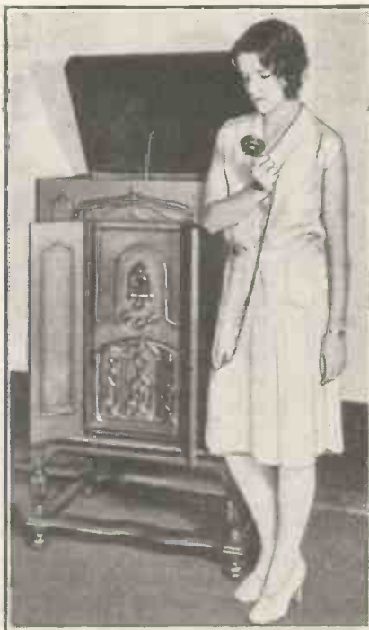
An American super-het radio-gram which includes the necessary devices for making your own gramophone records.
