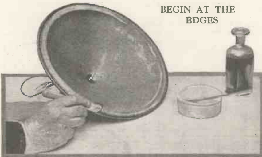
It is desirable to start applying the dope to the edges of the cone so that the fabric will tighten up evenly.
