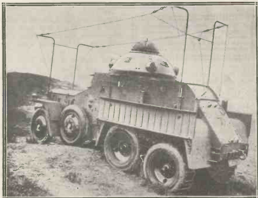
An eight-wheeled armoured car which is able to keep in wireless touch with its headquarters whilst spoiling the landscape around it.
