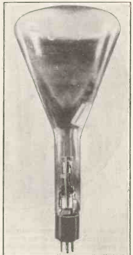
The tube used at the receiving end; the image appears on the fluorescent screen on the end. It is called an "Oscillite."
