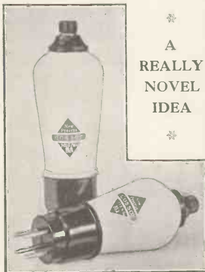
Two Cossor screened-grid valves, one battery and one mains type, which are shielded by being sprayed with a metallised paint which is in electrical contact with the filament.
