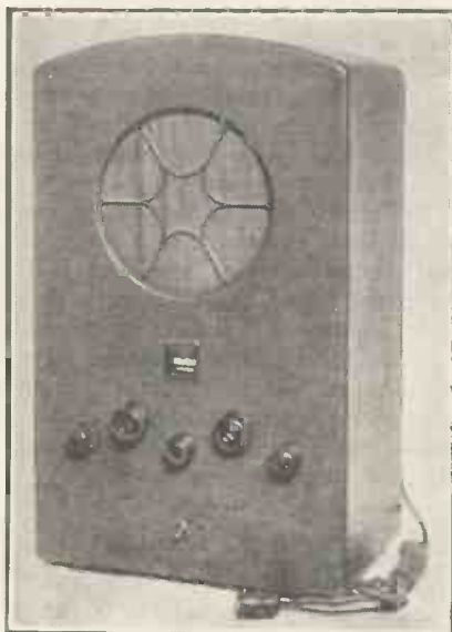
Here you see the front of the three-valve model. The controls, starting from the left, are: Volume, trimmer, wave-change switch, tuning condenser, and reaction, with the "on-off" switch at the bottom.
