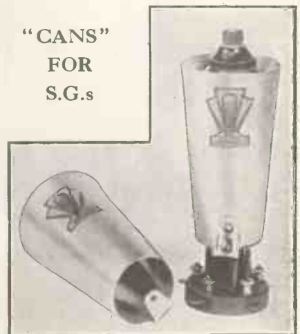
Special Six-Sixty aluminium shields which fit round the valve, and have a tab on the bottom through which one filament pin passes, thus earthing the shield
