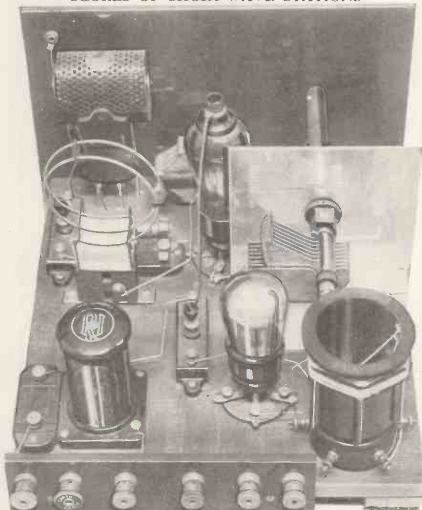
This general view of the adaptor, which enables one to hear scores of stations, provides a good idea of the layout and the simplicity of the wiring. The valve in the foreground is the oscillator; the S.G. detector can be seen partly hidden by the small metal screen.
