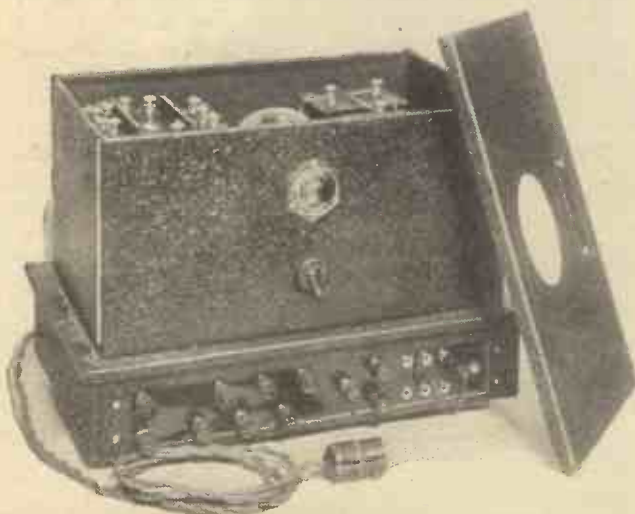
This unit gives H.T., L.T., and grid bias from A.C. mains.
