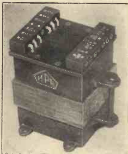
Much of the success of a unit depends upon the efficiency of its individual components. Here is a well-designed mains transformer.
