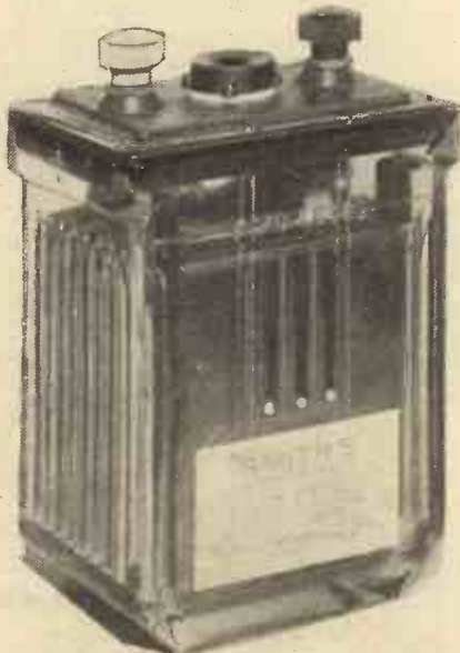
One of S. Smith & Sons' "indicating" batteries. Note that the three indicators are "sunk," showing the battery is very badly run down.
