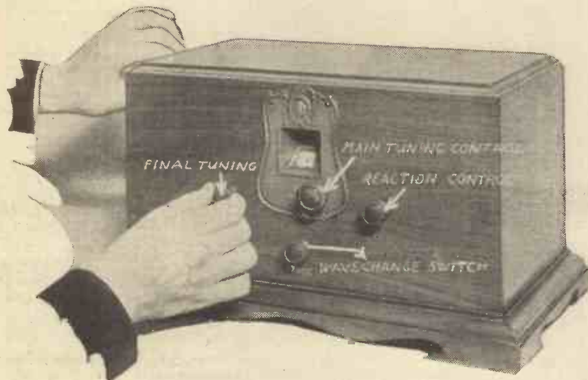
The "Ekco S.G.P. Three" is very easy to handle, and on this photograph our artist has indicated the use of the various controls.
