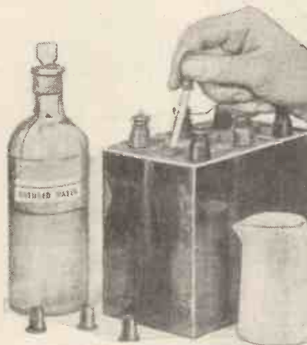
Topping-up the accumulator must always be done with distilled water.
