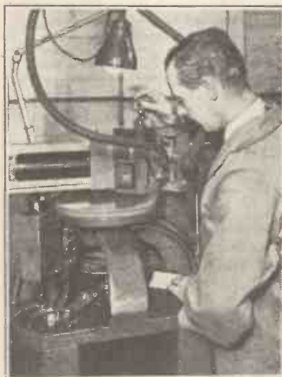
Trimming and polishing the wax "blank" before it is sent to the recording studio.
