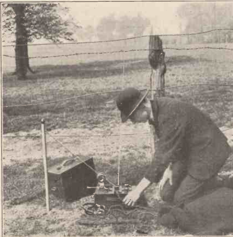
A wire fence makes quite a good aerial. The metal stake is stuck into the ground in order to obtain the necessary earth connection.
