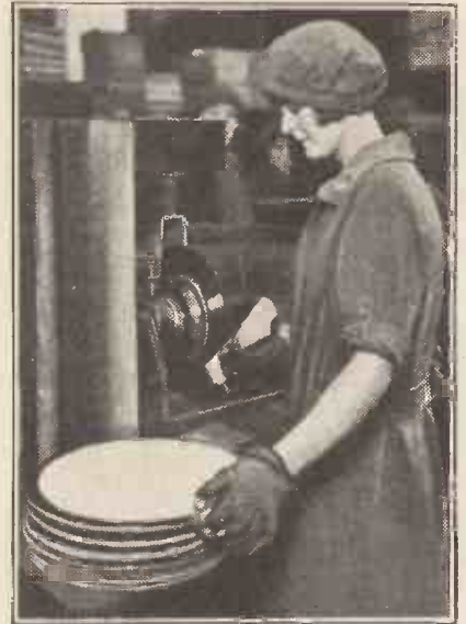
Polishing the edges of Columbia records after they come from the steam presses.
