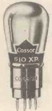
The super-power valve has the advantage of large grid swing, while the ordinary pentode "has it" on magnification, losing on the grid swing very considerably.
