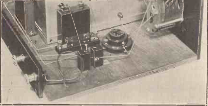
The “aerial end” of the set is extremely simple. Note the use of entirely standard coils.
