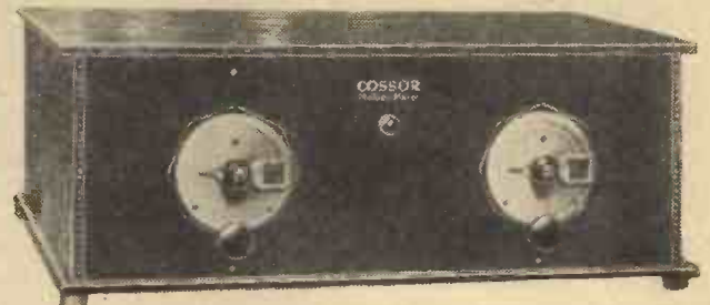
The "wave-change" switch figures on the front of the panel of the "Melody Maker," the "on-off" switch being at the back of the set.
