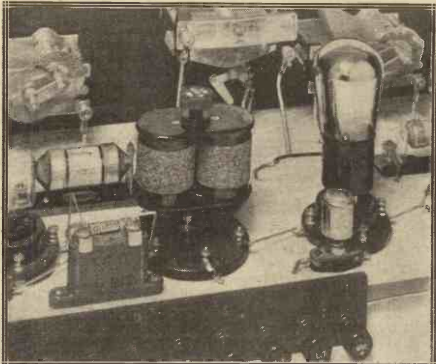
Radio receivers are becoming more and more simple to construct and operate. Self-neutralising valves, fieldless coils, examples of which are seen above, screened-grid valves, and other examples of the four-electrode variety, are tending to make for an economy and efficiency of working never before experienced.
