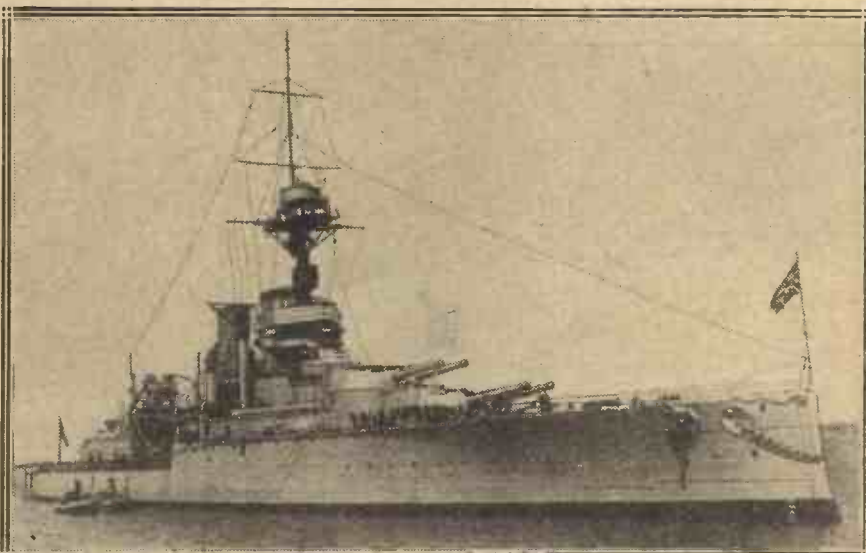
The above photograph depicts H.M.S. "Centurion," formerly a battleship and now converted into a target ship controlled by wireless. Without a single man on board her, she steers and manoeuvres in accordance with the marvellous machinery in her control room. The vessel automatically obeys the wireless instructions given by an officer on board another warship, even though the latter is miles away.
