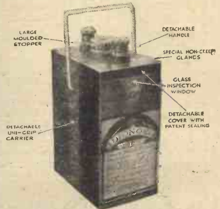
A Dionoid accumulator with its special features illustrated.
