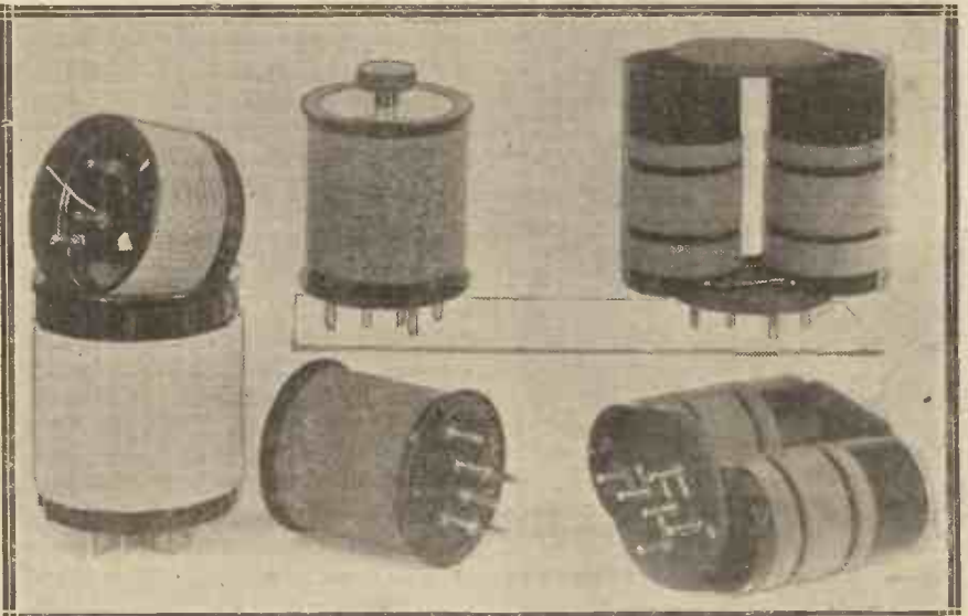
Modern tuning coils vary a great deal in design. In binocular coils, for instance (right), the windings are in opposite directions, in order to limit the coil's magnetic field
