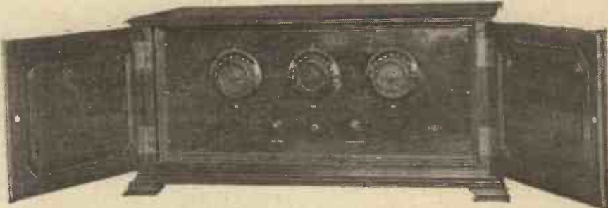
Many of the commercial sets now on the market include provision for the use of "pick-ups," and this Geophone four-valve receiver has a special plug-and-jack arrangement so that the set can be used with the gramophone.
