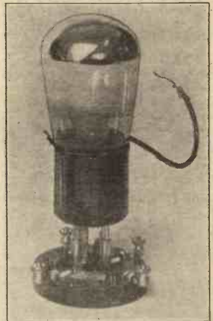
The tetrode has assisted in solving the problem of stability in H.F. circuits as exemplified by the screened-grid valve. This photograph shows another valve having two plates and two grids whose inter-electrode capacities are so arranged as to be self-neutralising.
