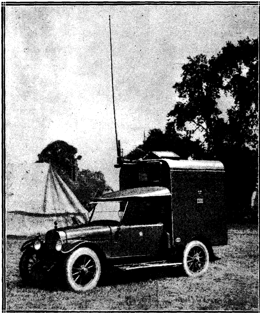
An Army Portable Wireless Station. Armoured cars are now being fitted with wireless, and the above photograph shows the Headquarters Car, with its mast erected.
