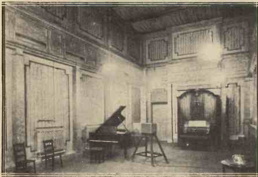
The latest studio (No. 7) at Savoy Hill, like its predecessors, employs draped walls and ceilings, echo effects being obtained by means of a special "echo" room.
