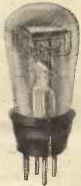
The new Marconi and Osram 410 valves are similar in appearance to the valve illustrated here, having a flat plate and long filament.
