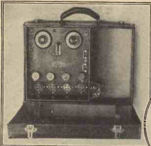
The Levis 4-valve portable shown above is contained in a normal-sized leather attache case and incorporates the same circuit as that employed in the 4A cabinet receiver. The whole set can be taken out of the case and used as an indoor receiver if desired. Including royalties, but excluding 'phones or loud speaker, the Levis portable costs £25.
