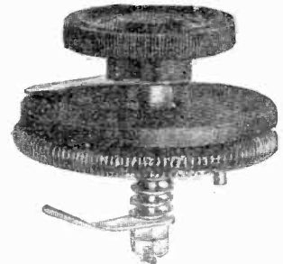
FILAMENT RHEOSTATS. With finished and lacquered brass bush for panel mounting. Resistance wire wound on insulating rod, thereby giving perfectly smooth adjustment. 2 or 5 ohms resistance 3/- each. 30 ohms resistance 3/6 each.
