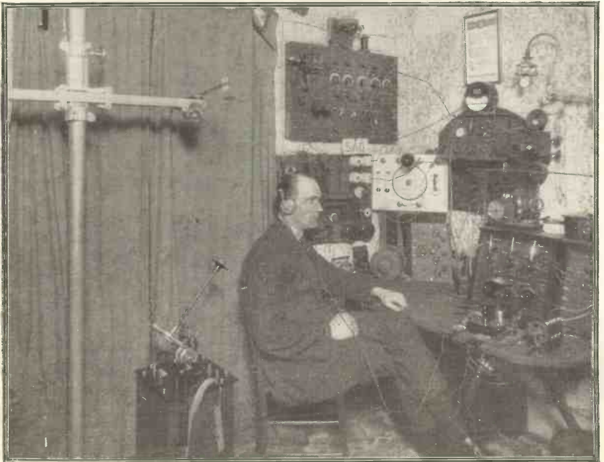
5 AQ, Mr. D. Douet's station at Putney. Mr. Douet has used Myer's receiving valves succesfully for transmission with 300 volts on the plate and 6 volts on the filament. The aerial current was .29 ampere.
