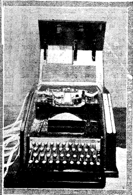
Above: The Kleinschmidt perforator, an ingenious apparatus which punches paper tape by the aid of a typewriter keyboard.
